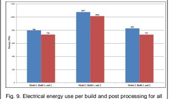
Fig. 9. Electrical energy use per build and post processing for all models
