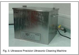
The Ultrawave cleaner uses a combination of ultrasonic waves, heat and a detergent to remove any excess support material used during fabrication without damaging the model itself.
