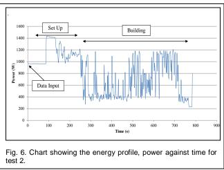
It can be observed form Figure 7 and 8 that at the point of the data input, there is a drop in the power as the machine processes the data that has been fed through the user interface of the computer, then, there is then a spike in the power as the machine begins to extrude material and build the part.
